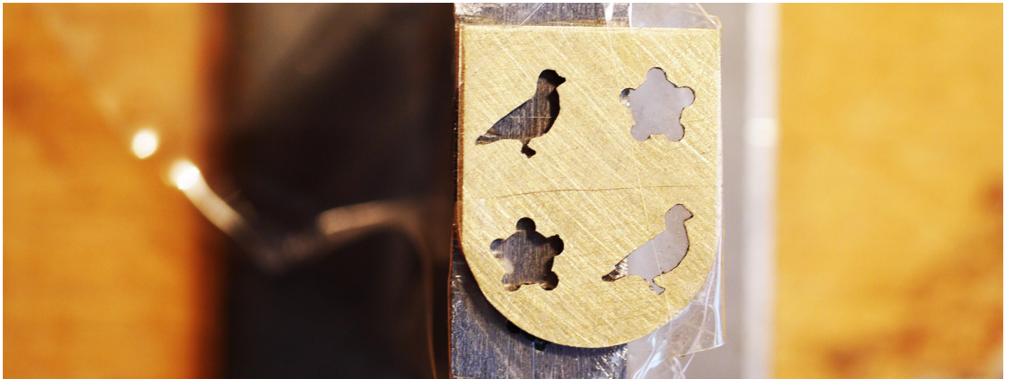
9 carat harden gold sheet prepared to receive and withstand the 4 shots
